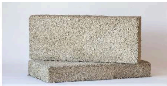
Fig 1.4 Mattone in calce e canapa ( greenplanner.it )
